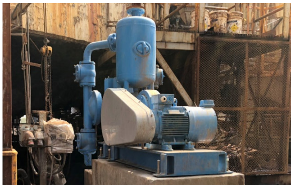
ABEL HM for jarosite filtration (AISI 316)
