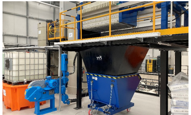
Dewatering automotive slurries with 800x800 mm (31.5x31.5 in.) filter plates: ABEL CM
