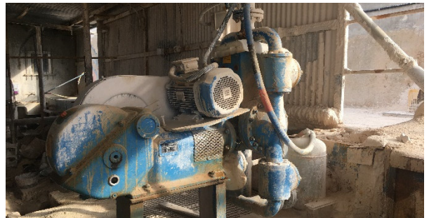
ABEL CM at 16 bar (232 psi), kaolin slurry dewatering
