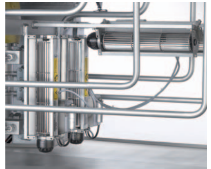
Tangential blowers to cool valve cylinders
