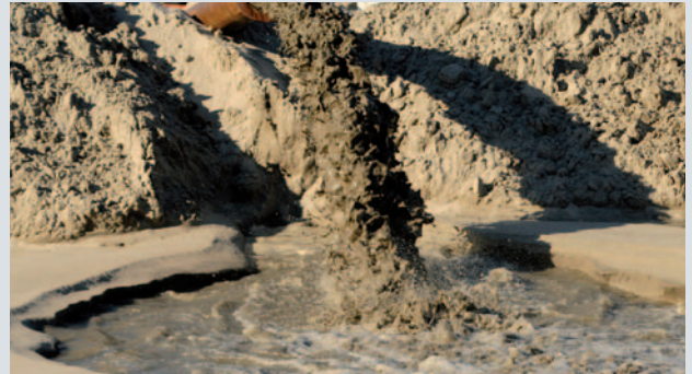
Silica slurry, 45 % solids concentration
