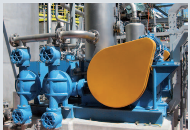
ABEL HMQ with duplex stainless steel wet ends for autoclave feed
