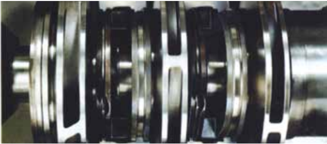
Staggered impeller vane tips reduce pressure pulsations at vane passing frequency.
