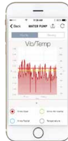
Trending Trend vibration, temperature, & kurtosis to monitor any changes in the equipment operation.
