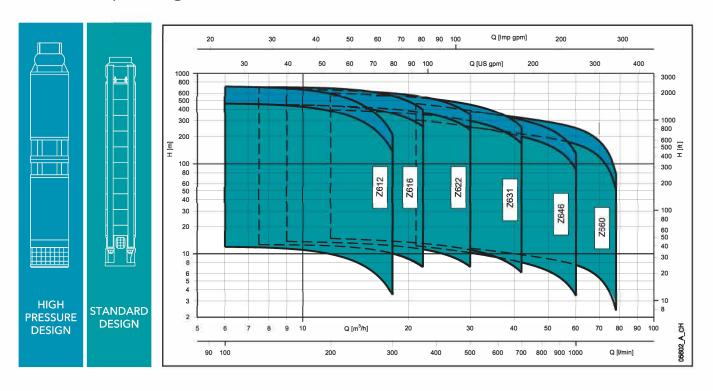
Z6 series operating characteristics at 60 hz.
