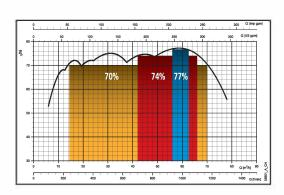
All the new Z6 series pumps offer a superior efficiency and therefore all points selected between 14 m³/h and 70 m3/h have always efficiency equal to or higher than 70% with a max efficiency of 77% within the overall Z6 range.
