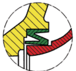
Wear ring in operation
