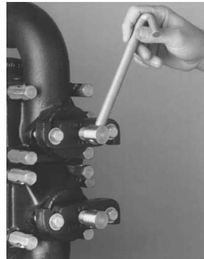
Figure 1: Loosening locking knobs
