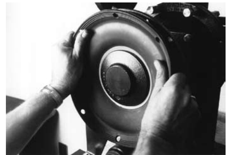
Figure 7: Align diaphragm holes with chamber holes
